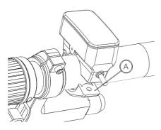
With the screw B (M3\*10 hexagon socket screw) tighten the display into position, torque requirement: 1N.m.
